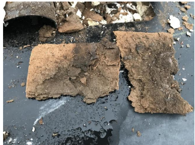
Figure 45: View of deteriorated coverboard.
